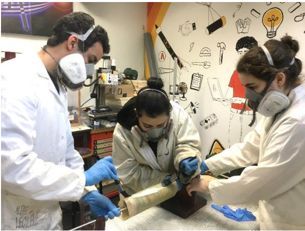
Figure 88, Realization of fiberglass envelope
